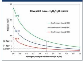
**Figure 3:** Condensation of the 125-280 Solution<sup>™</sup> during the Dynamic H2O2 exposure step for a 50 lb load at 26°C.
